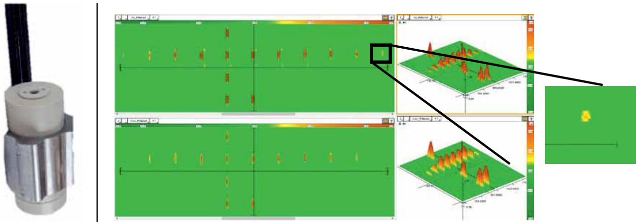
Fig. 6 : Left: Picture of a fuel rod probe assembly for PWR. Right: Typical data display from fuel rod probes – axial and transversal C-scan. 11 indications (cracks and pitting),
