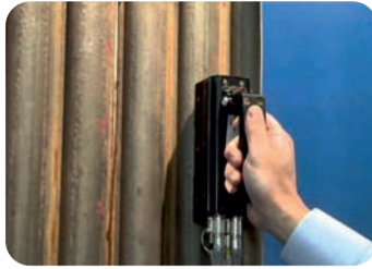
Thickness Mapping Of Boiler Tubes With EMAT
