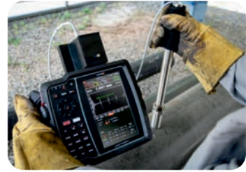
High Temperature Thickness Gauging With EMAT
