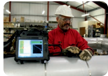
Corrosion Under Insulation By PECT
