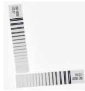
Figure 3 : Arrangement of Duplex wire IQIs for evaluation of detector Basic Spatial Resolution (SR b ).
